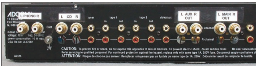
PHOTO 5: The rear panel with new input and output connectors and a new ground post.
