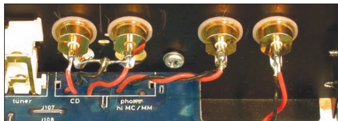
PHOTO 4: New CD input jacks are shown on the left, along with phono jacks on the right. The twisted-pair leads to the left phono input jack are soldered to the bottom of the PC board.
